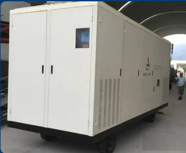
Controlled-atmosphere control cabinet
